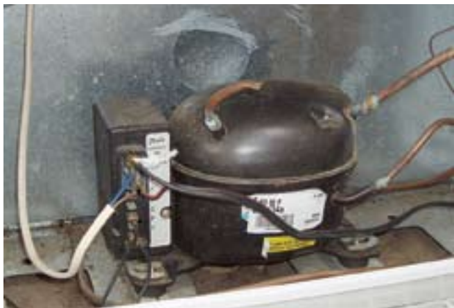
An efficient Danfoss compressor and lots of insulation combine to make an energy-saving freezer.
